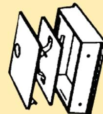
Some heating appliances require an air vent or brick to ensure safety and efficiency of operation, and to comply with ADJ and SBR.
